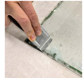
22. Cleaning the glass with a razor blade and glass cleaner
