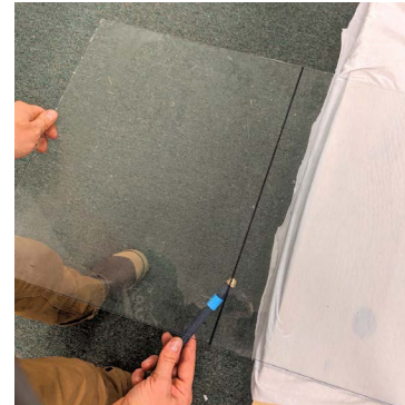
30. Tapping the underside of the glass to help it break
