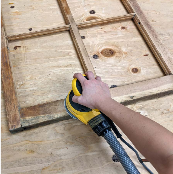
16. Giving the flat surfaces a light sand with an orbital sander
