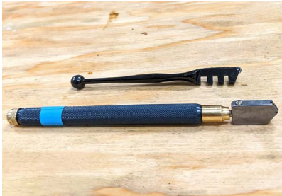
27. The glass cutter on the top is an inexpensive one that can be found at most hardware stores, though does not work as well as the one on the bottom with a carbide cutter and oil feed
