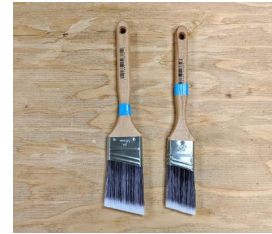
44. High-quality brushes with an angled chisel tip
