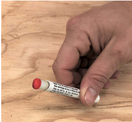
2. The red tip shows that lead is present in the painted sash
