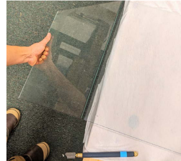
29. Breaking glass over the edge of the table
