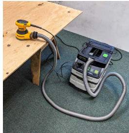
18. Orbital sander hooked up to a shop vac
