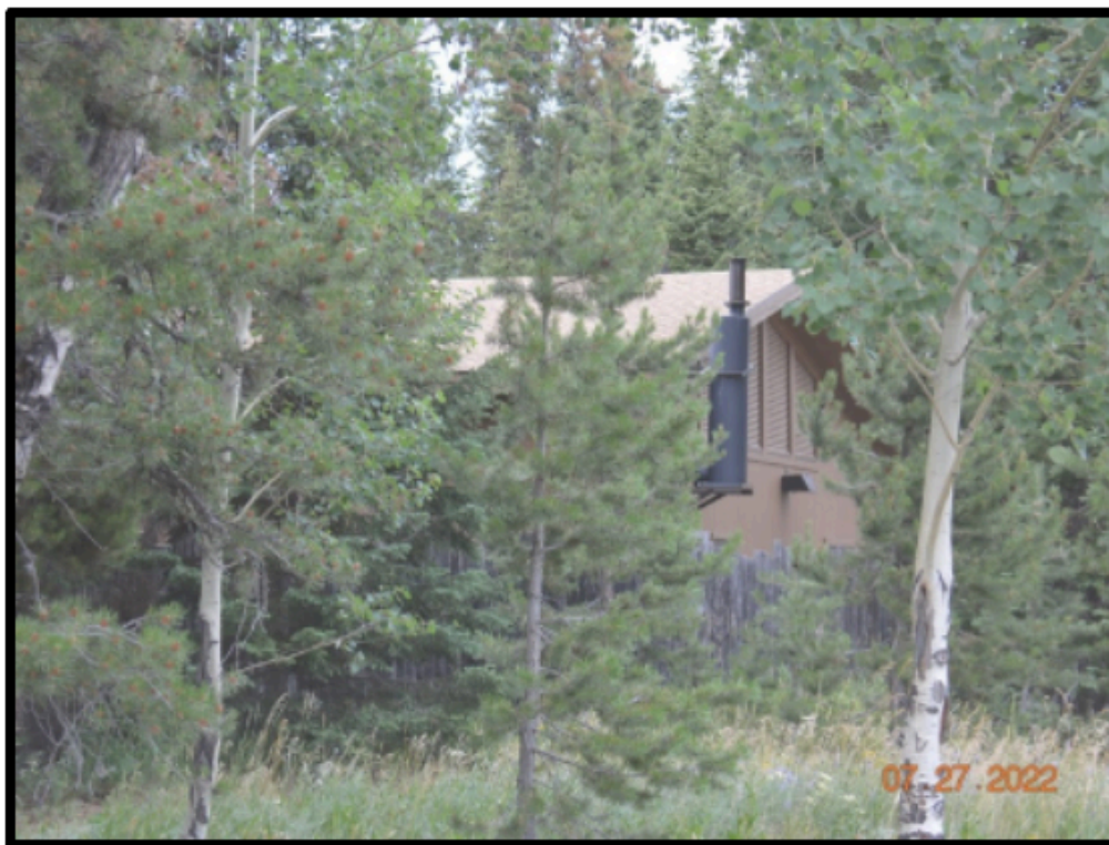
Figure 19. Horizontal and vertical continuity of vegetation in the immediate vicinity of a structure at an historic site. If the trees and shrubs contribute to its significance, mitigation and defensible space normally done in the WUI may not be appropriate.
